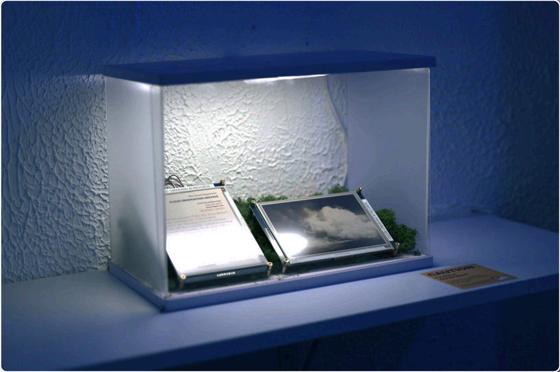
“Machine Cloud Observer” – The autonomous network device that sources and analyzes new cloud images from the internet (right screen), then generates formatted observation notes to be rendered on the e-ink screen (left screen).
